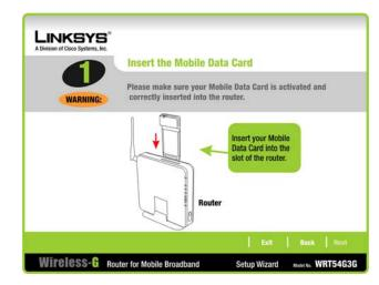
Figure 5-3: Insert Mobile Broadband Data Card Screen
